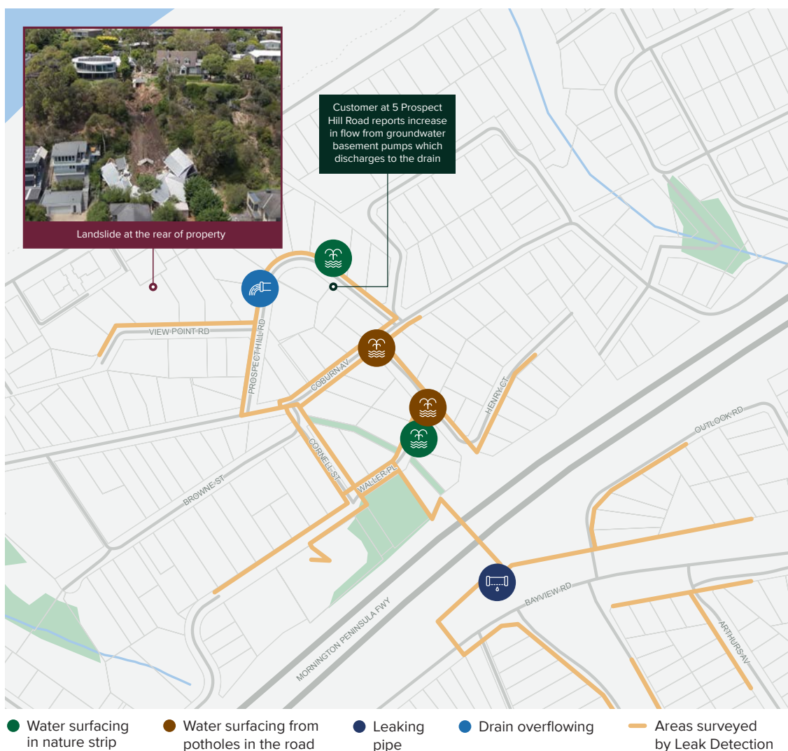
FIGURE 3.46: SCHEMATIC OF THE WATER NETWORK IN THE MCCRAE AREA ANNOTATED BY MR SWAIN. 781
