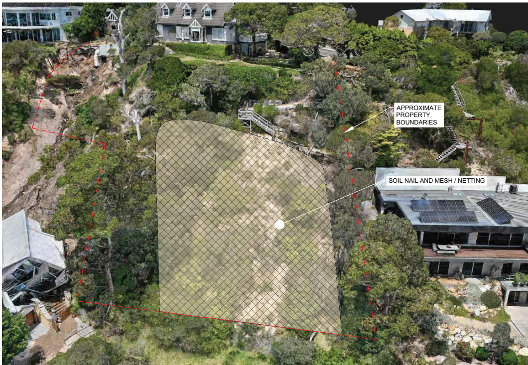
FIGURE 5.7: OBLIQUE VIEW OF SOIL NET DESIGN FOR WEST GULLY OF 10–12 VIEW POINT ROAD. 73
