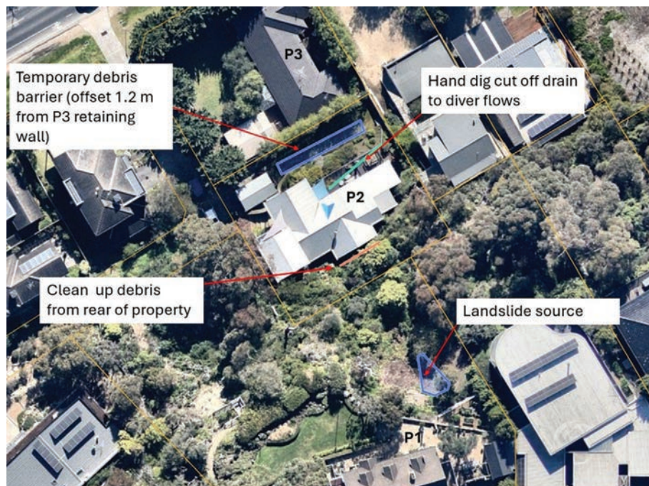
FIGURE 3.36: AERIAL PHOTOGRAPH ON WHICH MR POPE MARKED WHERE CERTAIN ACTIONS WERE TO BE TAKEN BY THE BORGHESES AND THE MORANS. 608
