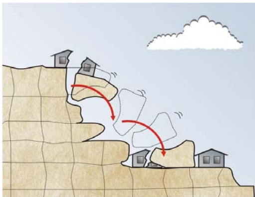
Figure 1 - Failure of an undercut block
