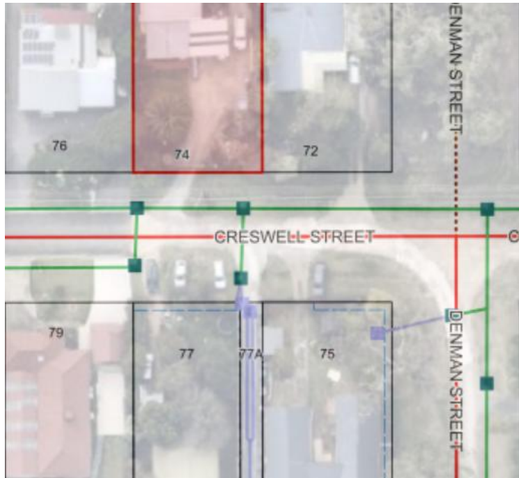
Figure 15 - Extract from Council's GIS system showing the area of the western addition of Creswell Street with existing drainage infrastructure, including drainage pipes and pits in green.
