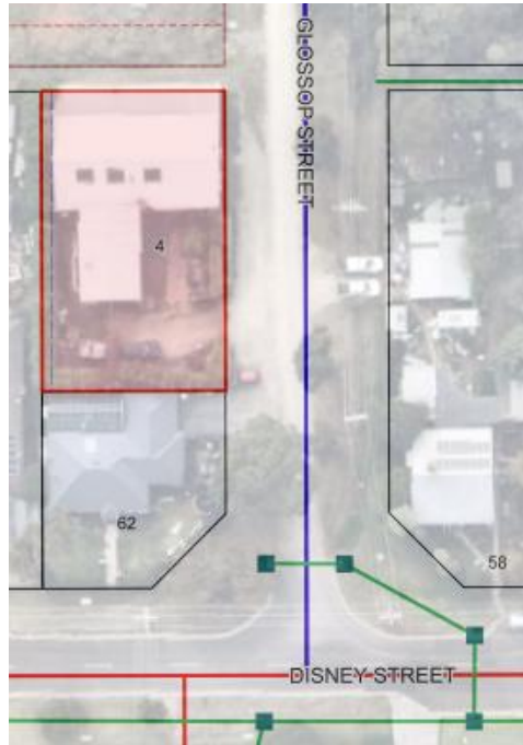
Figure 09 – Extract from Council's GIS system showing Glossop Street with existing drainage infrastructure, including drainage pipes and pits in green and indicative open channel drainage in blue.
