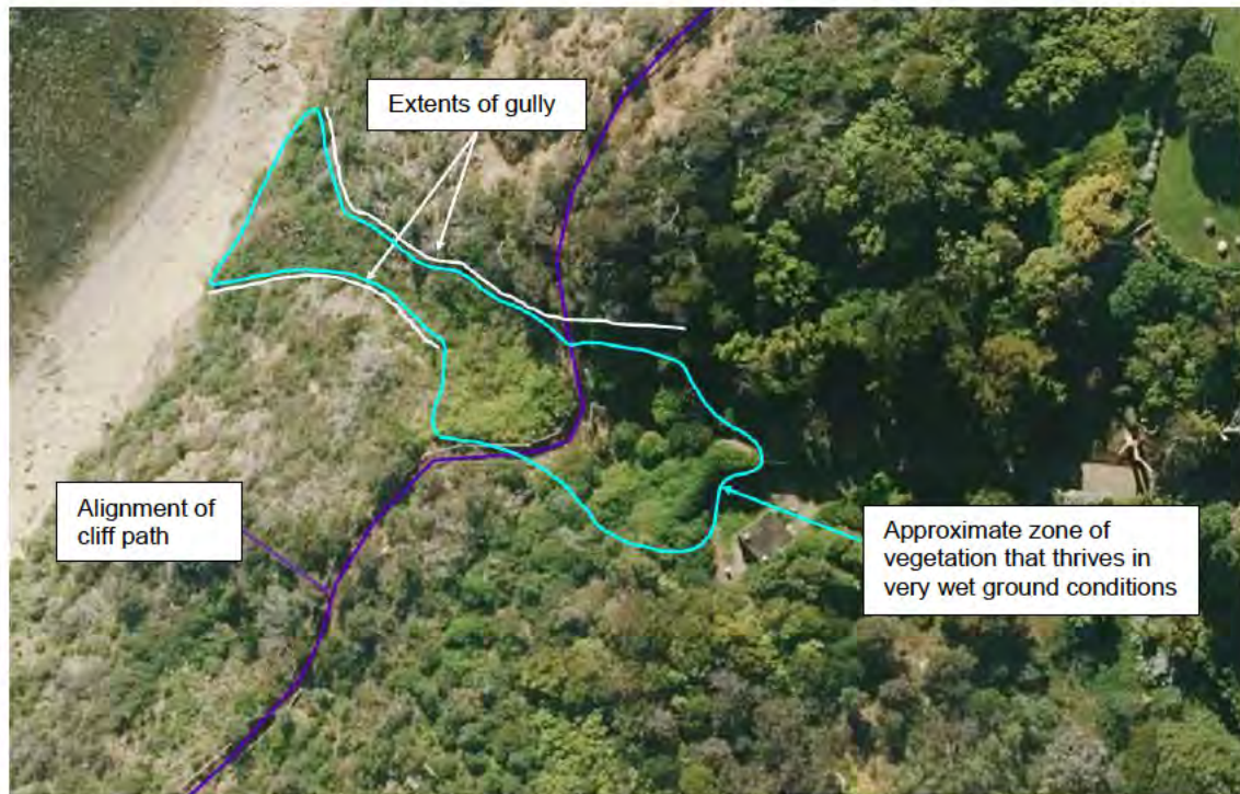
Figure 3-7 – Aerial image of a historic natural drainage gully in the mid-section of the path
