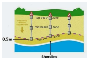
Figure 1. Visual depiction of transects and quadrants for beach litter auditing, each square is 1 x 1 metre and is searched for an allotted time of 5 minutes at the top beach, mid beach and tide line.
