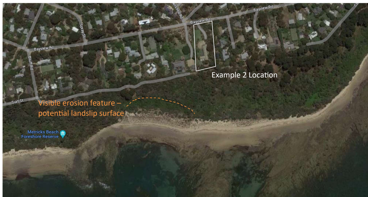
Figure 11 Example of potential landslip feature within coastal hazard zone
