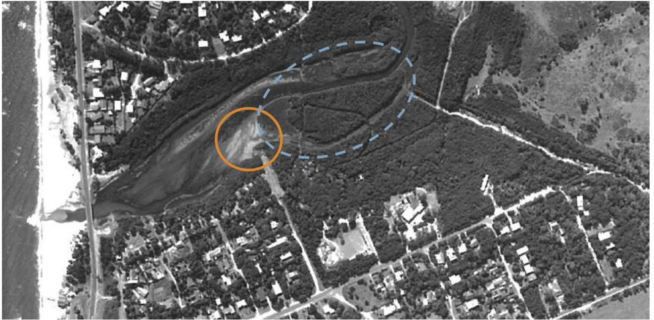
Figure 13. April 1977 historical aerial imagery (courtesy MPSC) – orange circle identifying area at the end of Henley Avenue – absence of defined bayhead delta. Main bayhead delta on Balcombe Creek indicated in blue circle.
