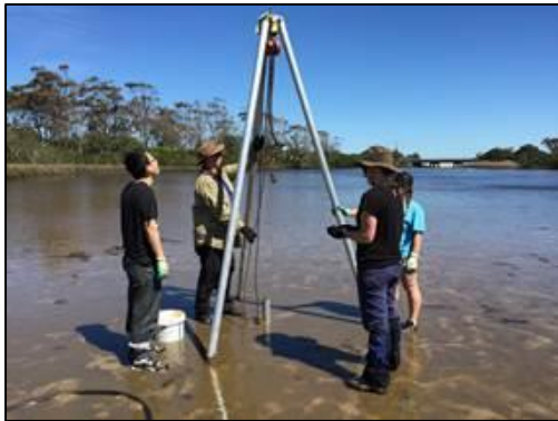
Figure 6. Vibrocoring in Balcombe Creek estuary
