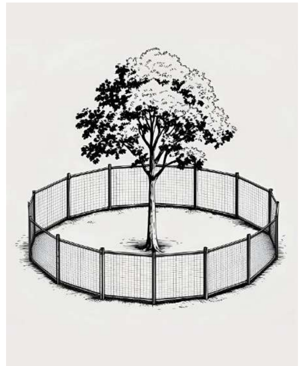
Figure 6.1. Illustrative example of a fenced tree protection zone (TPZ)
