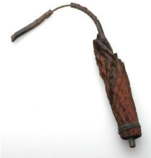
Figure 18: Section of 1870s Tasmanian submarine cable. 49
