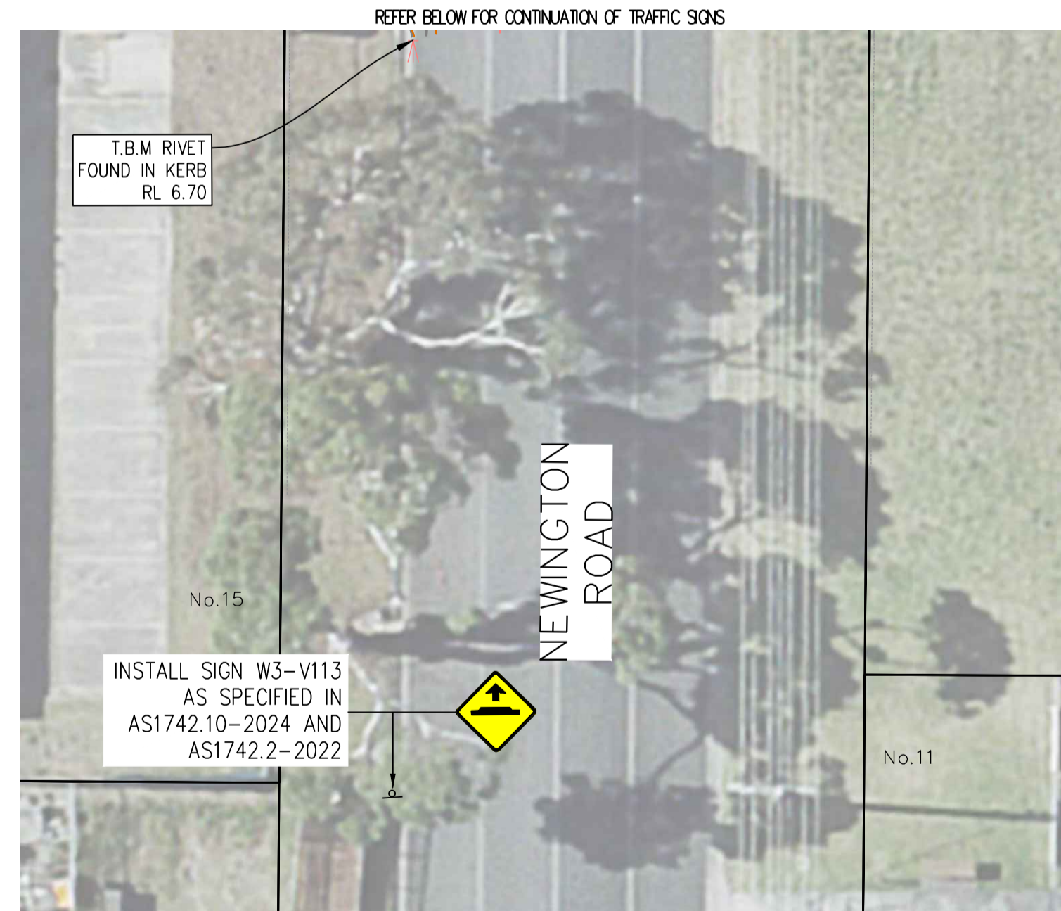
SIGNAGE AND LINEMARKING PLAN NEWINGTON ROAD
