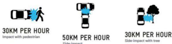
Figure 6 – Survivable impact speeds for different crash types
