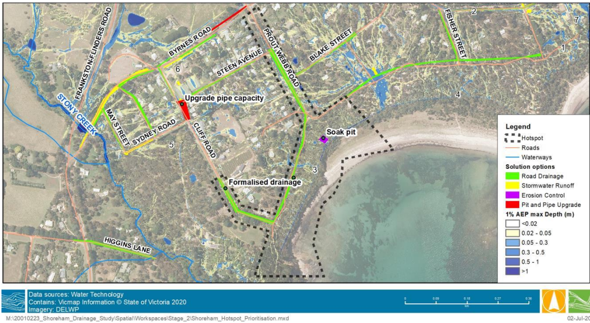
FIGURE 6-8 HOTSPOT 3(A AND B) - ISSUES AND CATEGORISED SOLUTION
