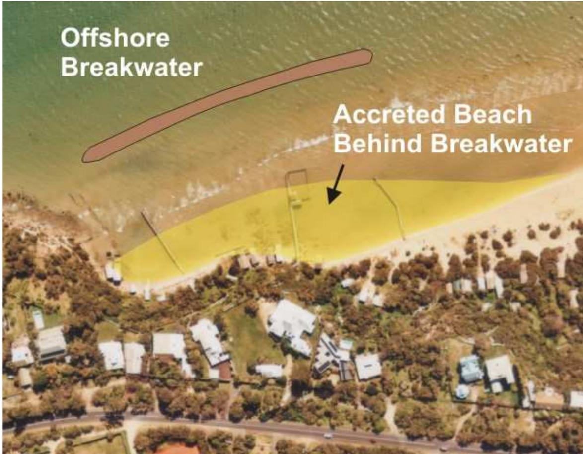
Figure 5.4: Offshore breakwater and accreted beach
