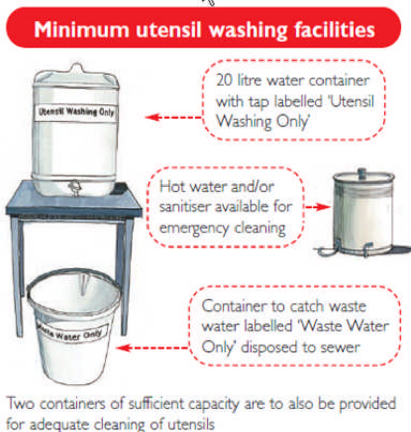
Figure 2 – Cleaning Facilities for Temporary Food Premises
