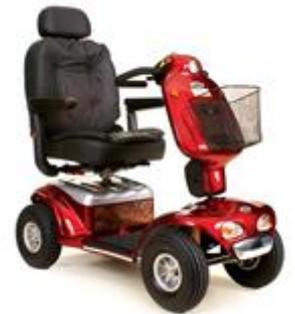
In general, electric scooters have a maximum speed of less than 10 kph. They are activated by a simple throttle, operated by the fingers, which controls both speed and braking. Steering is via a variety of types of handlebars that operate in a similar fashion to push bikes or motor bikes. They come with varying equipment levels depending on the level, from twin headlights, blinkers, visibility flags, even independent suspension, down to basic machines with simple controls.
